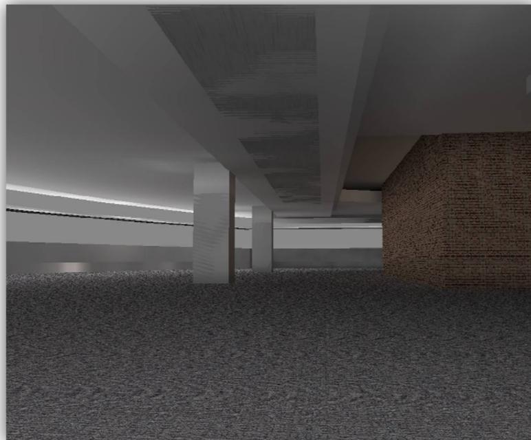
*Fig 9: Third floor indirect light distribution from light shelf at north east wall*
