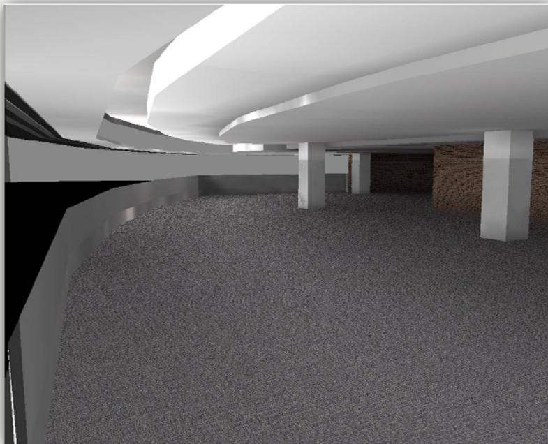
*Fig 7: Second Floor indirect light distribution from light shelf*
