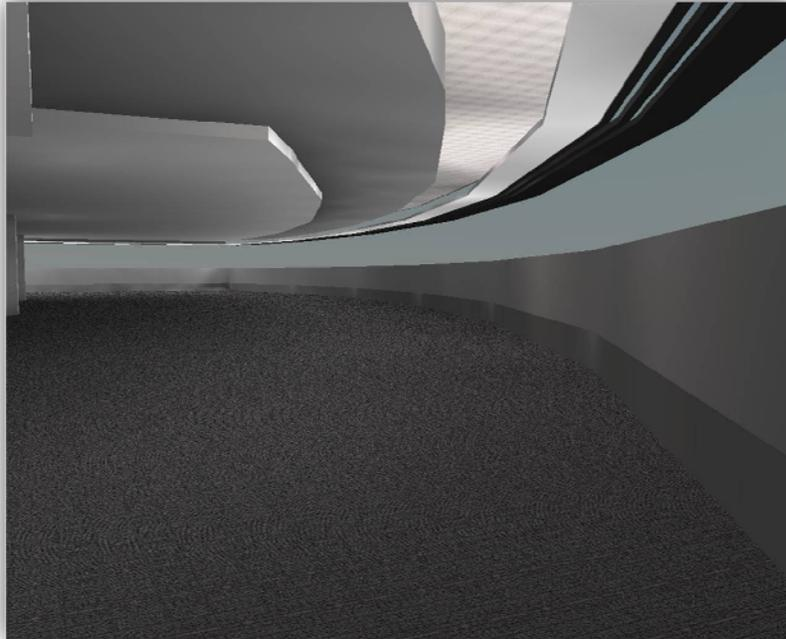
*Fig 8: Third floor indirect light distribution from light shelf*
